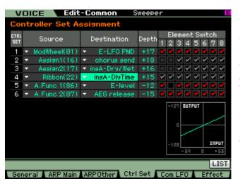
\_And then set the CONTROL TYPE = SCRATCH. \_If you assign a controller (your favorite) to the DELAY TIME, you will be able to create the same effect as having a movable playback head (like on the 'Echoplex'). The Echoplex was a classic tape recorder delay unit with multiple playback heads and a slide control to move one of the heads in real time.
